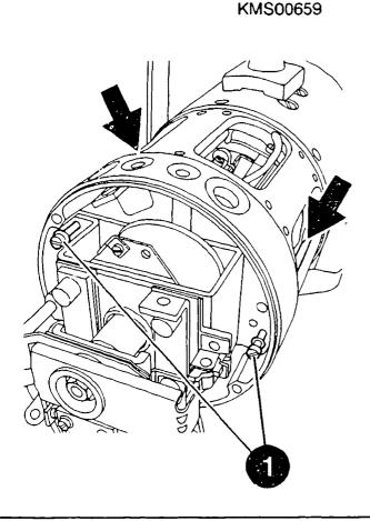
ASSEMBLING STARTING-MOTOR SOLENOID WITH CONTROL RELAY
